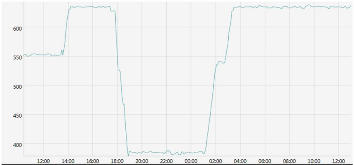
Figure 15. What a slag sheading load drop looks like.
