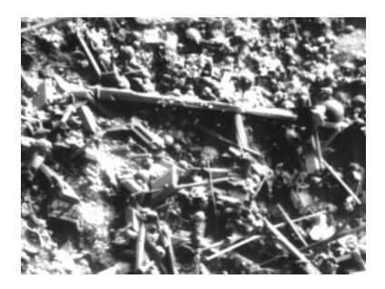
Figure 3. Crystals of CaSO4 bonding flyash together.
