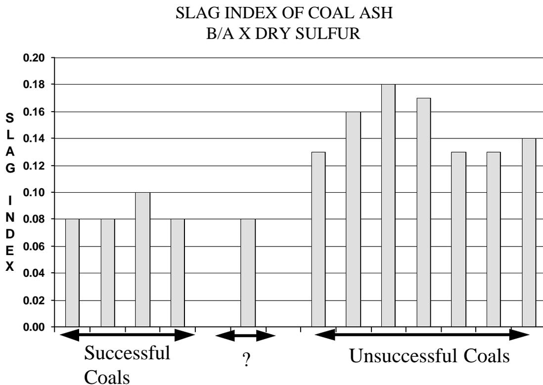
**Figure 6.** Slagging Index,  $R_s$  for coals by successful/unsuccessful categories, ? is coal that had some problems, but not as severe as unsuccessful coals.
