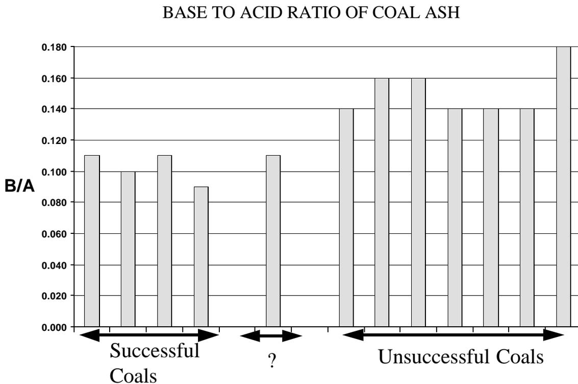
**Figure 5.** Base to acid ratio, B/A for coals by successful/unsuccessful categories, ? is coal that had some problems, but not as severe as unsuccessful coals.
