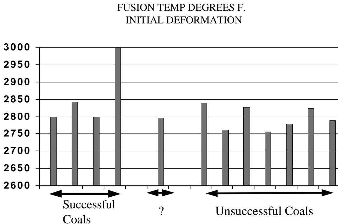
**Figure 1.** Initial deformation temperature for coals by successful/unsuccessful categories, ? is coal that had some problems, but not as severe as unsuccessful coals.
