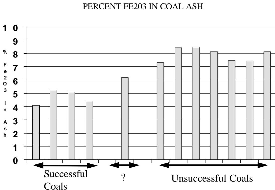
**Figure 3.** Iron oxide (Fe<sub>2</sub>O<sub>3</sub>) levels in coal ash by successful/unsuccessful categories, ? is coal that had some problems, but not as severe as unsuccessful coals.
