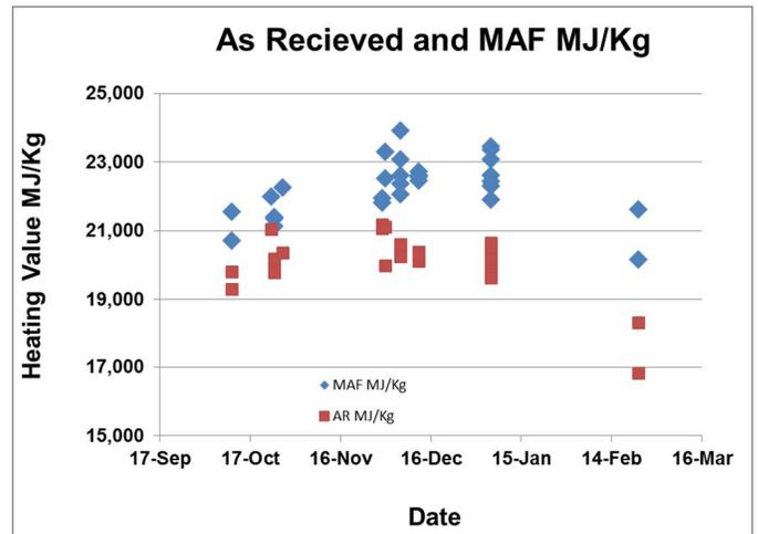
Fig. 9 The loss of both MAF and AR heating value of TW fuel in storage
