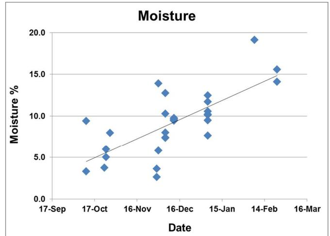
Fig. 8 Shows increase of moisture content of TW fuel during storage.
