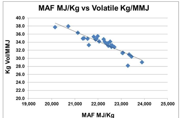
Fig. 6 Relationship between MAF heating value and volatile content; showing loss of volatile content with increased torrefaction.
