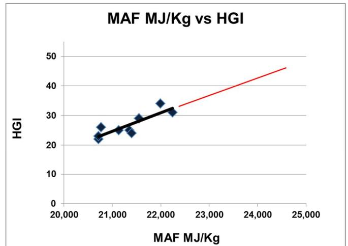
Fig. 5 Relationship of MAF heating value vs HGI for test burn samples showing extension of trend to evaluate where MAF heating value would be for a minimum HGI of 40.
