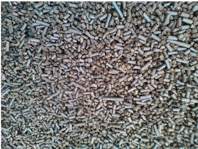
Fig. 1 Uniform colored pellets from commercial facility using ground wood as feedstock and then pelletizing.
