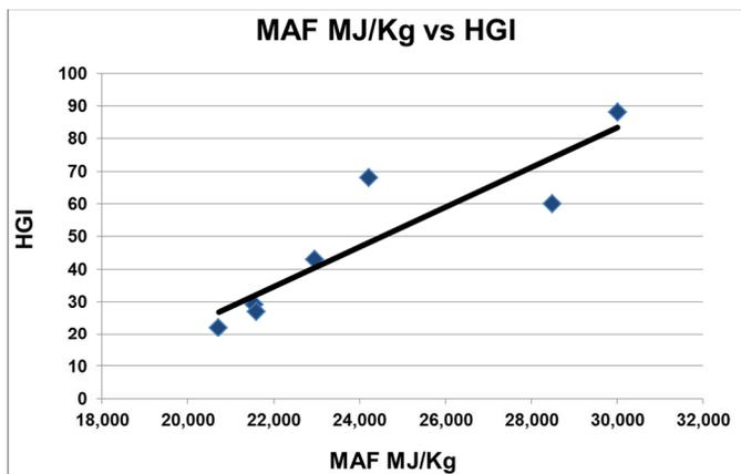
Fig 4. Relationship between MAF heating value and HGI over a wide range of torrefaction.
