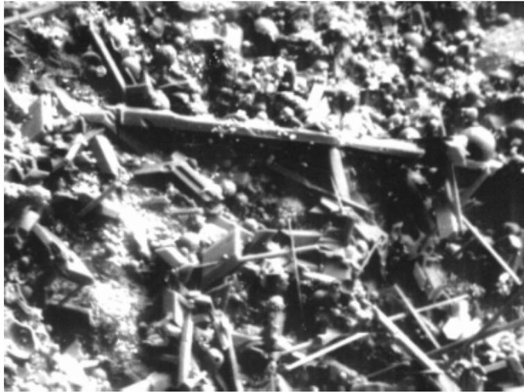
Figure 3. Crystals of CaSO<sub>4</sub> bonding flyash together.
